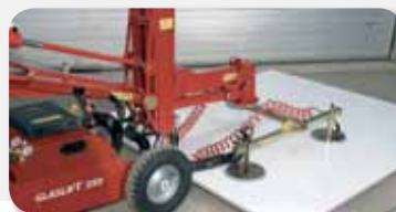
Hydraulic horizontal lifting arm pick-up
